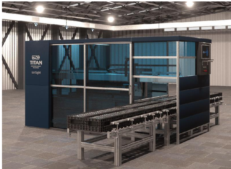
Figure 2. Titan's IonSight™ inspection platform. This rendering illustrates Titan's most recent system engineered to perform automated, in-line 'Digital Teardowns' of battery cells using advanced ultrasound tomography.
